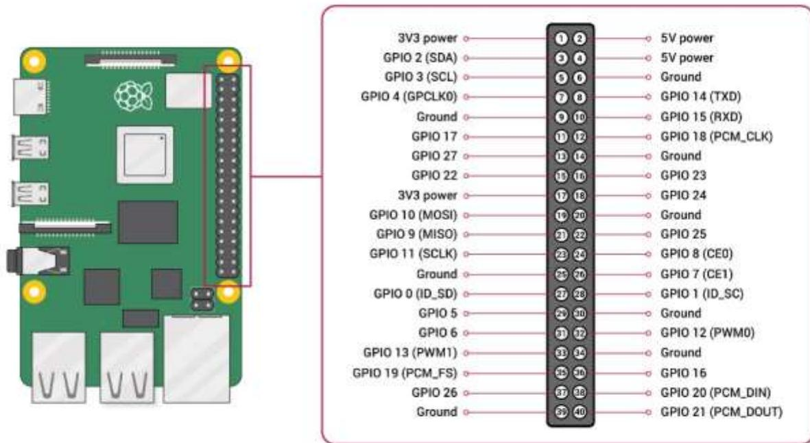
Figura 12.4 GPIO Raspberry Pi
